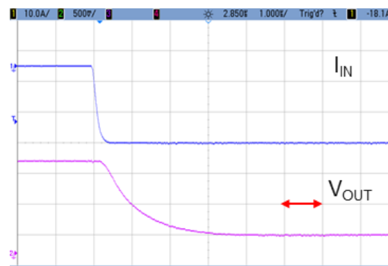
Figure 9. Rise response waveform (left), fall response waveform (right).
