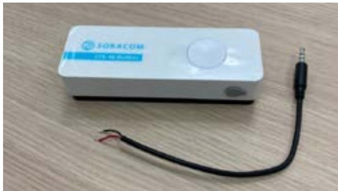
At the heart of this project, I used the Soracom LTE-M Button. The button is a simple, yet highly versatile device that can send click events from anywhere in the world to the cloud. You can check out my unboxing and initial setup of the button [here](#)! In this project, the button sends the signal to the webApp.
