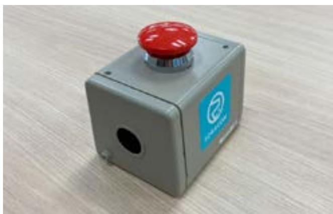
I used a switch interface to both house the electronics and cables, and provide some visual flare! This isn't really necessary, since you can use the built-in button on the micro:bit, or make a custom casing from cardboard and aluminum foil if you're crafty.
