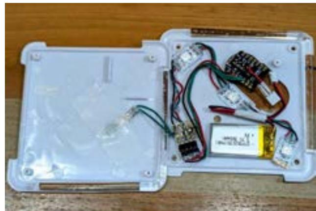
The part where the Seeeduino XIAO ESP32S3 is exposed was the original location of the device's battery. This does mean that the lid just barely closed, though the prototype was used in an open state during the exhibition to enable charging and debugging; for our initial-build purposes, this was acceptable.
