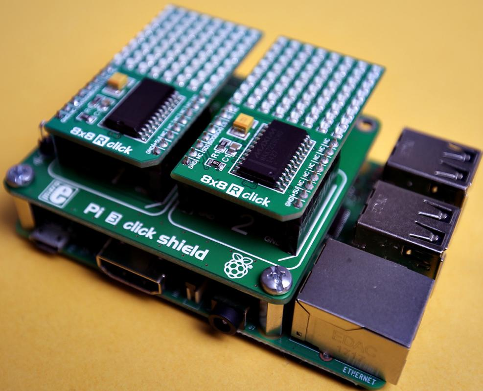
To demonstrate an example of the SPI protocol used on the Raspberry Pi, we've plugged two 8x8 R click boards™
