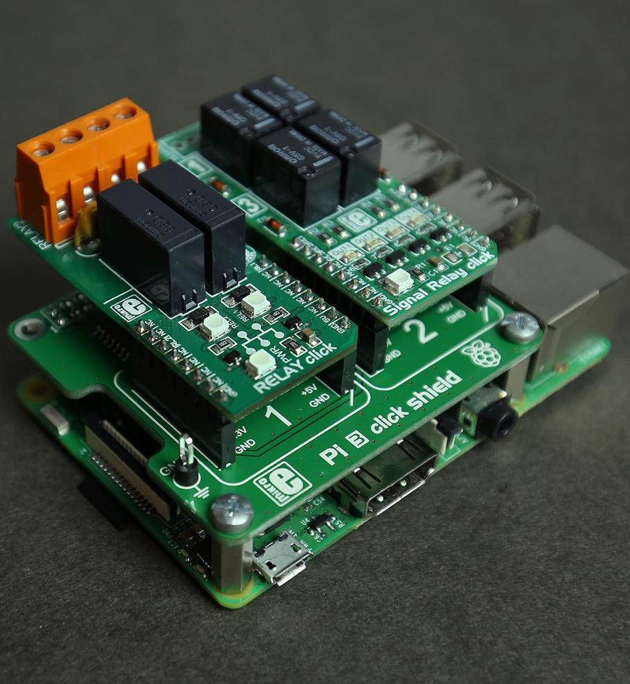
To show an example for GPIO pins used on the Raspberry Pi we've plugged two click boards™, Relay click and Signal Relay click, into the mikroBUS™ sockets which are a part of the Pi 3 click shield.
