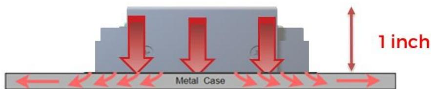
c. Semi-Potting: Facilitates heat dissipation while safeguarding PCBA components from moisture and dust.
