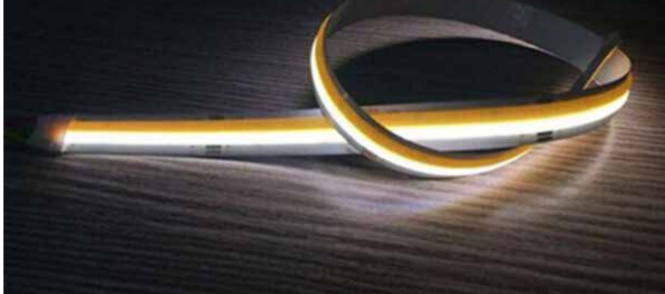
Figure 4: Consisting of unpackaged LEDs mounted on flexible substrates, COB light strips , like this one from American Bright, offer high brightness output. They're available in monochrome, white light, dual white light and addressable RGB LED formats.
