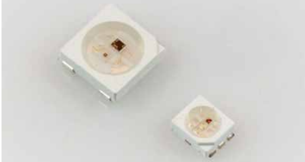
Figure 1: These RGBHC addressable LEDs from American Bright incorporate red, green, and blue dies, as well as an IC into a single surface mount package. They're available in a variety of sizes and form factors, and as an AEO-Q102 qualified part.
