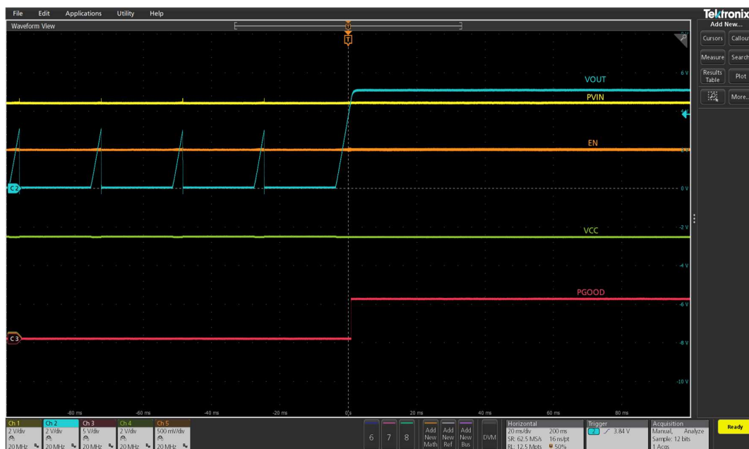
Figure 13 Over-current protection and auto-recover to 3A (Ch1:PV IN , Ch2: V OUT , Ch3: PG, Ch4:V CC , Ch5: Enable)
