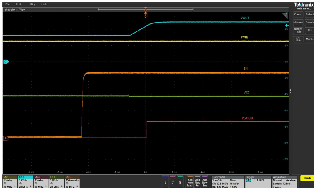
Figure 12 Startup into pre-bias. Max 70% of Vout. (Ch1:PV IN , Ch2: V OUT , Ch3: PG, Ch4:V CG Ch5: Enable)
