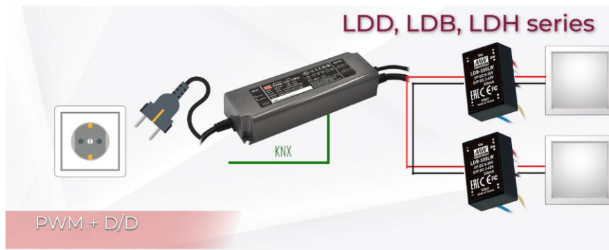
Figure 7 KNX direct driver for driving constant current LED panel lamp together with DC/DC converter
