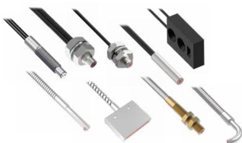
Fiber optics use an amplifier and fiber optic cables. The amplifier contains all of the electronics and the fiber optic cables act as light pipes to send the light wherever is needed. Because the fiber optic cables can be bent and routed, they can be used in space-constrained areas, harsh environments, and any other application with remote sensing requirements. The variety of sensing heads on the fiber optic cables adds to number of problems that can be solved.
