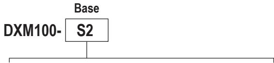
S2 = Modbus slave device for valve control, SDI-12 data collection for MultiHop wireless networks or wired networks
