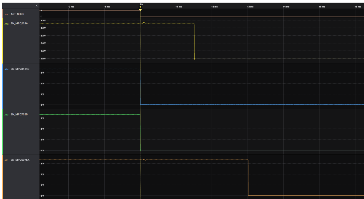
Figure 35: MPQ79700FS Enable during Power-Off Sequence
