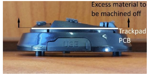
Figure 5.8 Side profile of proposed trackpad layout on ear piece structure
