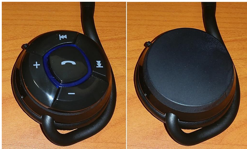
Figure 5.17 The original tactile button solution vs. the new gesture trackpad implementation
