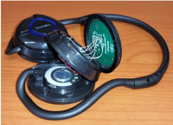
Figure 5.15 Connection wires soldered and tucked into earpiece
