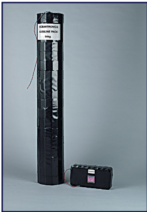
Delivered by helicopter near the North Pole, Oceantronics' GPS/ice buoy measures wind, temperature, sunlight, ice thickness, and GPS location of icebergs. The device was originally powered by a large battery pack (left) using 380 alkaline D cells (54 kg). The redesigned battery pack (right) substituted 32 bobbin-type LiSOCl 2 D cells and four hybrid layer capacitors (HLCs) to reduce size and weight (3.2 kg).
