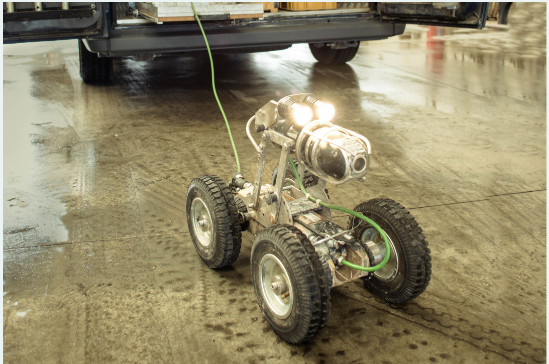
Figure 3: Improved sensors, autonomy, mobility and AI (allowing deep learning) is enabling inspection robots to replace humans, especially in hazardous or confined areas like inside pipelines or in storage tanks.
