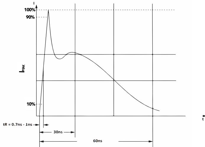
Voltage ranges from 4kV to 15kV for air discharge, and 2kV to 8 kV for contact discharge. It is this peak current that must be reduced in order to mitigate any ESDfailure. Transient voltage suppressors is commonly used in circuit design for ESDprotection.
