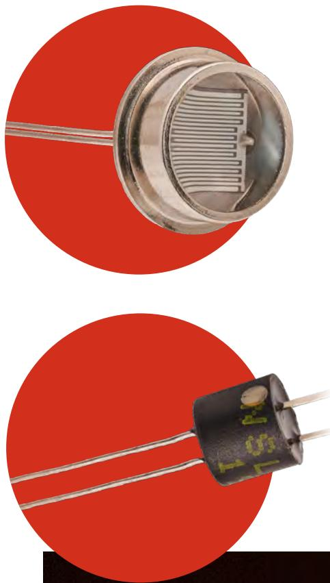
Light Dependent Resistors (LDR) measure visible light from 400 to 700 nm. The device resistance decreases as the light level increases with efficiency characteristics similar to the human eye. These LDRs are available in various resistance values and packages.
