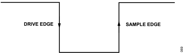
Figure 65. SPI Mode 3, SCLK Edges
