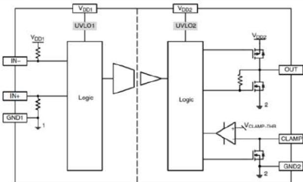
Figure 2. Simplified Block Diagram, NCD57090A/D/F
