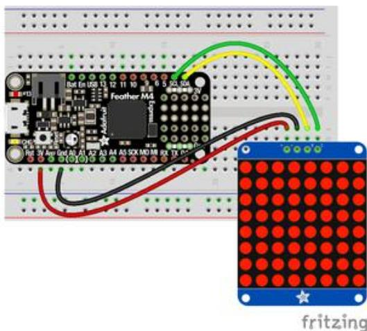
Microcontroller 3V to LED Matrix VIN
