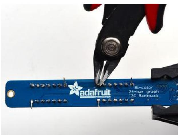
Once soldered, clip each pin. They're quite short and the pins are thicker than usual, so do this over/inside a trash bin so that the pins don't fly off and hit you or your pets.
