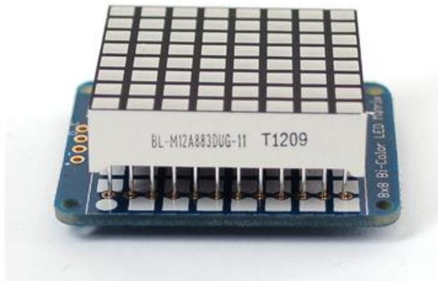
The matrix must be soldered on the correct orientation or it will not work! Check for the side of the matrix that has printing on it. Then look for the front of the PCB that has a circle instead of a square in the corner and line those up as shown on the left
