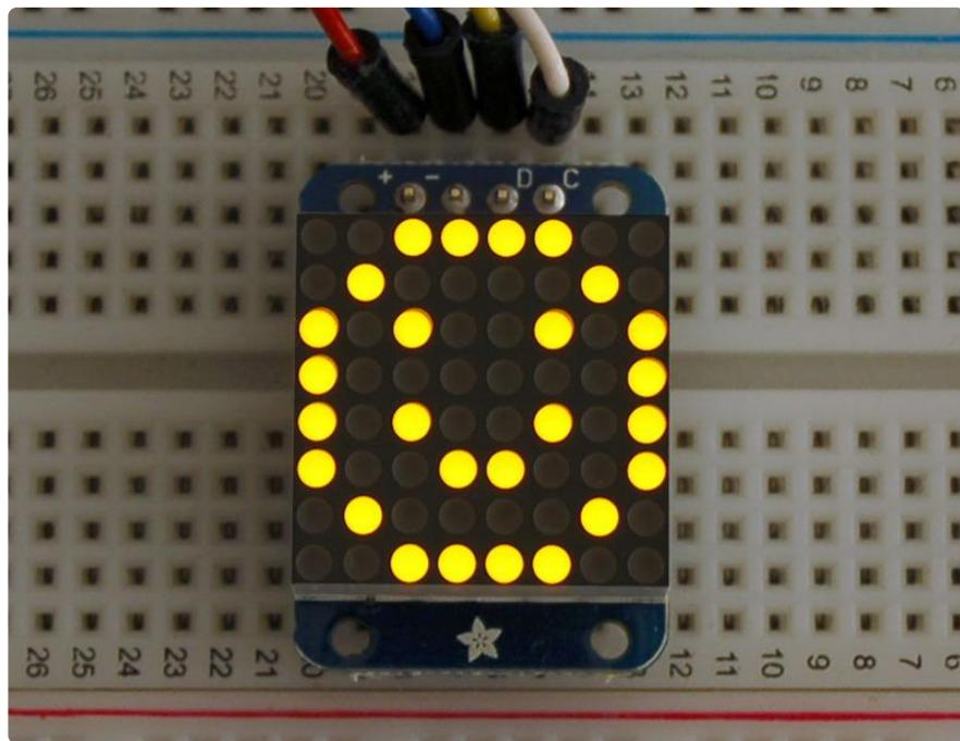
Once you're happy that the matrix works, you can write your own sketches. The 8x8 matrix supports everything the Adafruit GFX library - drawing pixels, lines, rectangles, circles, triangles, roundrects, and small bitmaps. [For more details check out the GFX page which will detail all of the GFX routines](https://adafru.it/aPx) (<https://adafru.it/aPx>).
