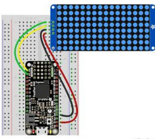
Microcontroller 3V to LED Matrix VIN
