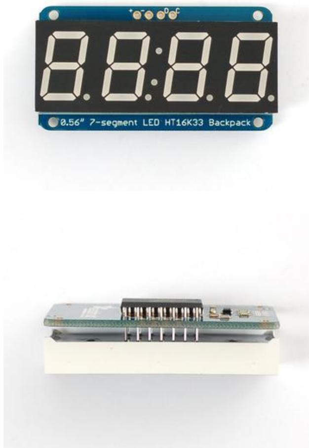
Remove the parts from packaging and place the LED matrix **OVER** the silkscreen side. **DO NOT PUT THE DISPLAY ON UPSIDE DOWN OR IT WONT WORK!!** Check the image below to make sure the 'decimal point' dots are on the bottom, matching the silkscreen.
