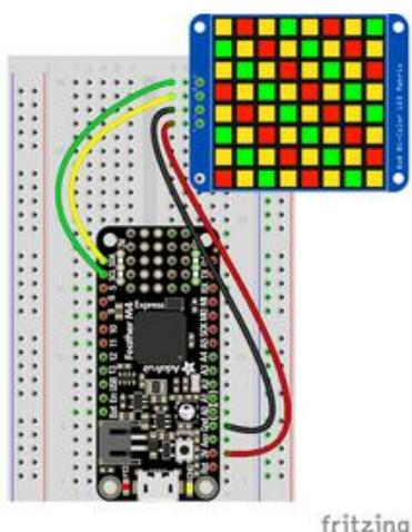
Microcontroller 3V to LED Matrix VIN
