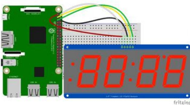
Raspberry Pi 3.3V to 7-Segment Display IO
