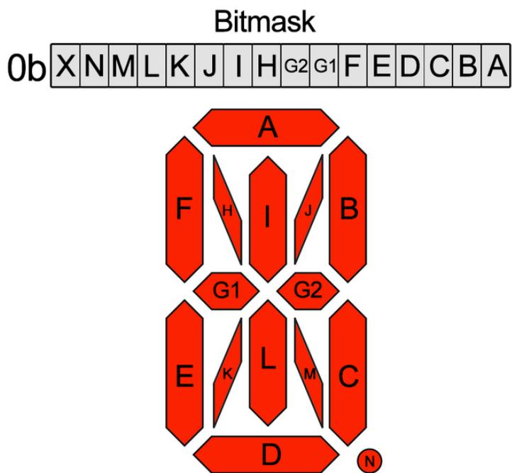
The bitmask is a 16-bit number that can be passed in as a single Hexadecimal, Decimal, or binary number. It can also be passed in as a list or tuple containing 2 separate 8-bit numbers. Here are some of the ways to set the digits. All of these different methods create a box with an X in the center:
