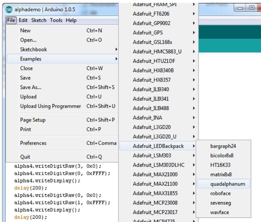
Upload to your Arduino, and open up the Serial console at 9600 baud speed. You'll see each digit light up all the segments, then the display will scroll through the 'font table' showing every character that it knows how to display. Finally, you'll get a notice to start typing into the serial console. Type a message and hit return, you'll see it
