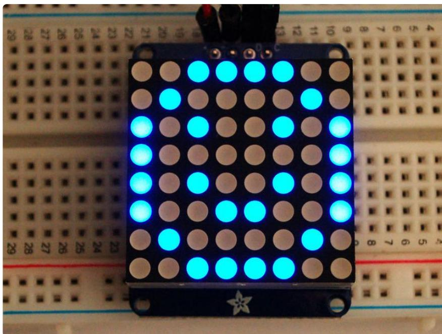
Once you're happy that the matrix works, you can write your own sketches. The 8x8 matrix supports everything the Adafruit GFX library - drawing pixels, lines, rectangles, circles, triangles, roundrects, and small bitmaps. [For more details check out the GFX page which will detail all of the GFX routines](https://adafru.it/aPx) (<https://adafru.it/aPx>).
