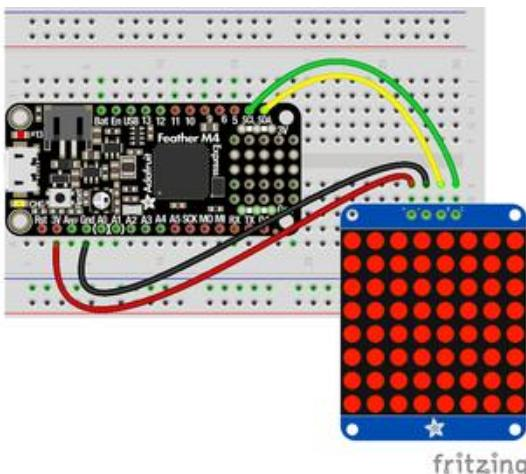
Microcontroller 3V to LED Matrix VIN
