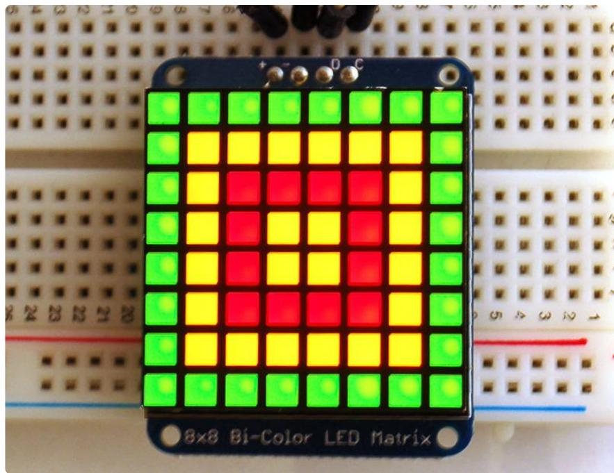
Once you're happy that the matrix works, you can write your own sketches. The 8x8 matrix supports everything the Adafruit GFX library - drawing pixels, lines, rectangles, circles, triangles, roundrects, and small bitmaps. [For more details check out the GFX page which will detail all of the GFX routines \(<https://adafru.it/aPx>\).](#)
