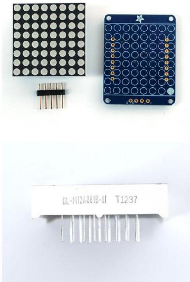
When you buy a pack from Adafruit, it comes with the fully tested and assembled backpack as well as a 8x8 matrix in one of the colors we provide (say, red, yellow or green). You'll need to solder the matrix onto the backpack but its an easy task.
