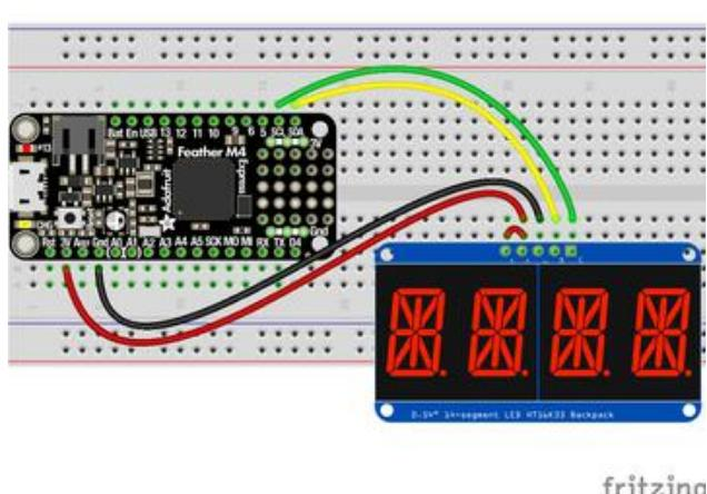
Microcontroller 3V to AlphaNumeric Display I2C VIN
