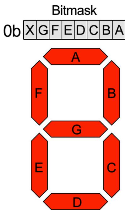
The bitmask is a single 8-bit number that can be passed in as a single Hexadecimal, Decimal, or binary number. This will use a couple different methods to display `8E8E`:
