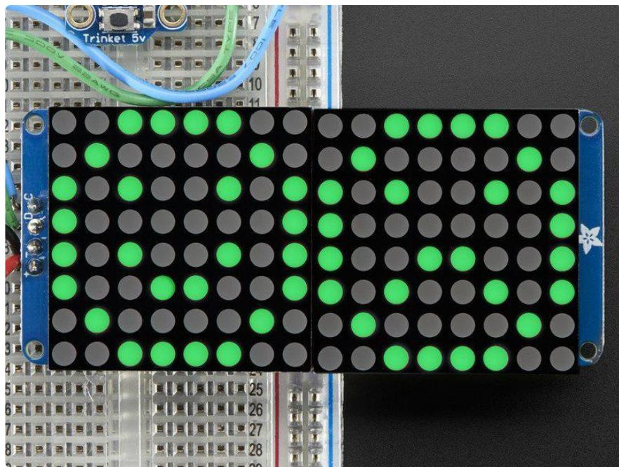
Once you're happy that the matrix works, you can write your own sketches. The 8x8 matrix supports everything the Adafruit GFX library - drawing pixels, lines, rectangles, circles, triangles, roundrects, and small bitmaps. [For more details check out the GFX page which will detail all of the GFX routines \(<https://adafru.it/aPx>\).](#)
