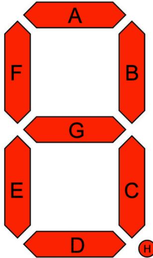
The bitmask is a single 8-bit number that can be passed in as a single Hexadecimal, Decimal, or binary number. This will use a couple different methods to display
