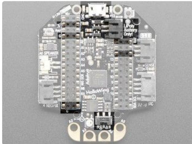
There's two ways to power your Hallowing. The best way is to plug in a 3.7/4.2V Lipoly battery into the JST 2-PH port. You can then recharge the battery over the Micro USB jack. You can also just run the board directly from Micro USB, it will automatically 'switch over' to USB power when that's plugged in
