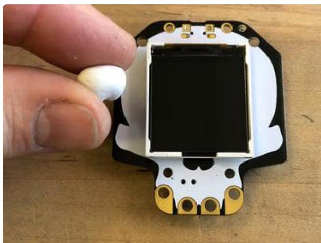
Roll the ball into a small cylinder and press up against one side of the board and screen.
