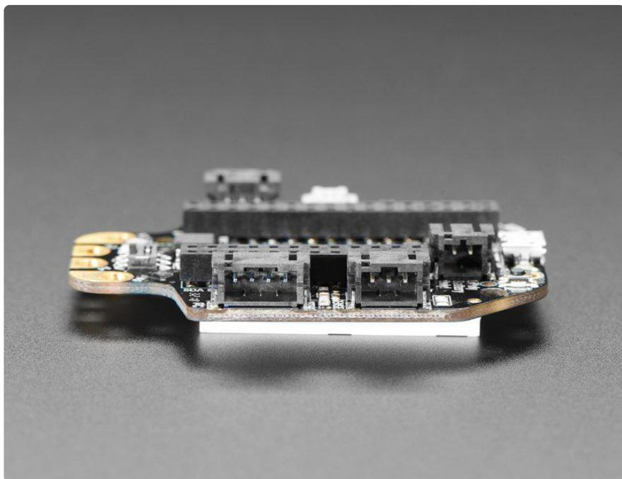
On each side of the Hallowing are JST-PH plugs for connecting external devices. The 3-pin JSTs connect to analog pins on the SAMD21, so you can use them for analog inputs. We label one for Neopixel and one for Sensors since we think most people will have one of each. The 4-pin JST connector connects to the I2C port and you can fit Grove connectors in it for additional hardware support.
