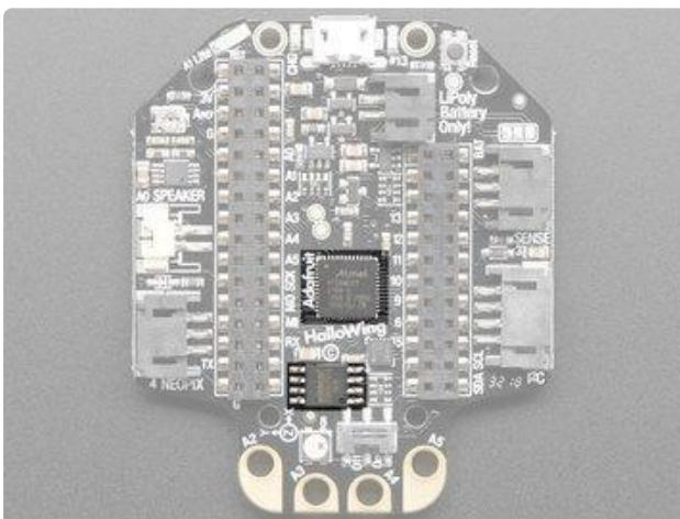
The main processor chip is the ATSAMD21G18 Cortex M0+ running at 48MHz with 3.3V logic/power. It has 256KB of FLASH + 32KB of RAM and can run Arduino or CircuitPython
