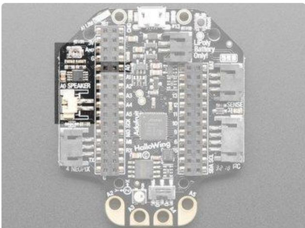
We have a mono 2 Watt class D audio amp connected to A0 - that's the DAC output on the SAMD21, so you can get 10-bit audio output, good for many simple sound effects or musical output. There's a small smt trimpot you can adjust if you want, but the default 50% setting is pretty good.
