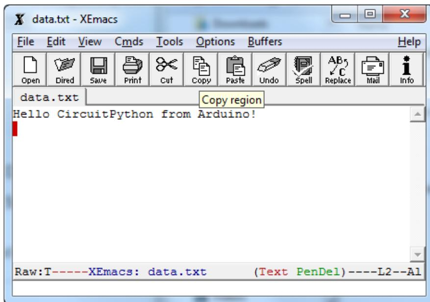
Once you have your Arduino sketch working well, for datalogging, you can simplify this procedure by dragging CURRENT.UF2 off of the BOOT drive to make a backup of the current program before loading circuitpython on. Then once you've accessed the file you want, re-drag CURRENT.UF2 back onto the BOOT drive to re-install the Arduino sketch!
