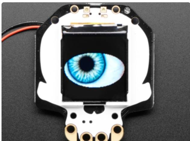
On the front is a 128x128 TFT. The TFT is connected to the SPI pins: SCK and MOSI (MISO is not connected)
