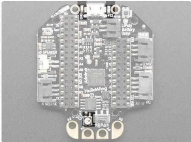
There are three LEDs - a red LED on pin D13, a CHG LED that will let you know when the battery is charging, and a NeoPixel on D8 (in Arduino) or `board.NEOPixel` (in CircuitPython)
