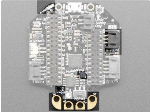
On the top there's a light sensor, connected to pin A1 - it's reverse mount so you can read light levels from the front.
