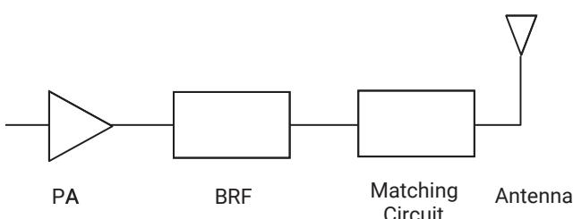
Harmonic rejection is usually performed by a LPF located after the PA, but the need often arises to suppress a spurious harmonic at a later stage of development or when the circuit is actually in production. In these cases an KAVX Accu-P® Thin-Film RF capacitor is the preferred solution.
