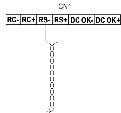
Sense lines should be twisted in pairs
