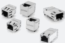
Integrated Connector Modules (ICMs) incorporate the ethernet signal magnetics used for filtering and isolation into the RJ45 connector housing to simplify your design, minimize overall PCB footprint, and enable excellent EMI performance.
