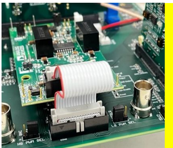
FIGURE 17: JUMPER SET TO CTRLR INPUT
