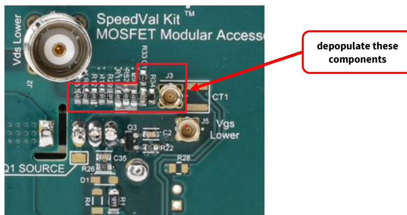
FIGURE 21: DAUGHTER CARD WITH SHUNT RESISTORS
