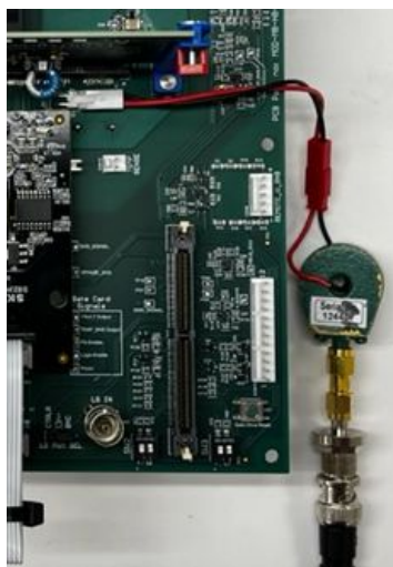
FIGURE 23: HIGH-BANDWIDTH CT CONNECTED TO CON11
