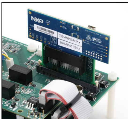
FIGURE 7: NXP CONTROL BOARD WITH INTERPOSER
