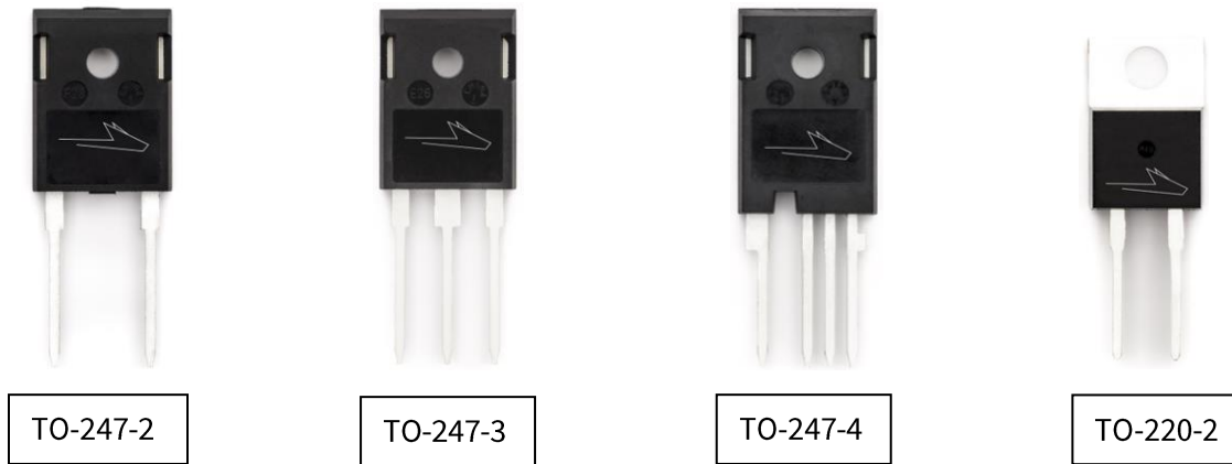
Figure 1: Through-Hole Package Examples
