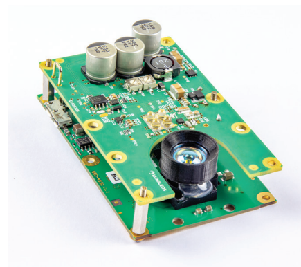
Melexis TOF evaluation kit with LUXEON IR Domed Line emitters
