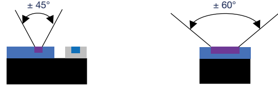
Fig. 8 - Field of View of Photodiode Horizontal (left) and Vertical (right)
