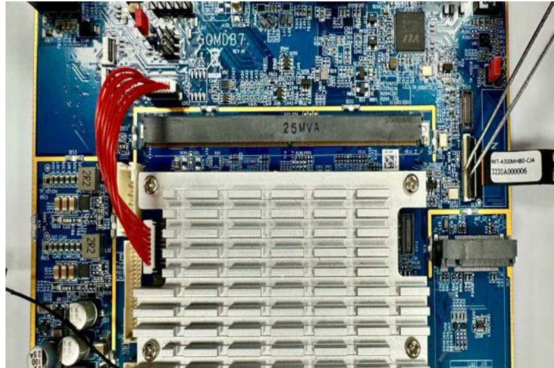
Figure 05: Lift the lock of the MIPI CSI connector 'CSI2'
