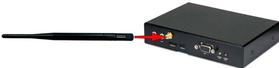
Figure 05: Installing the Wi-Fi antenna
