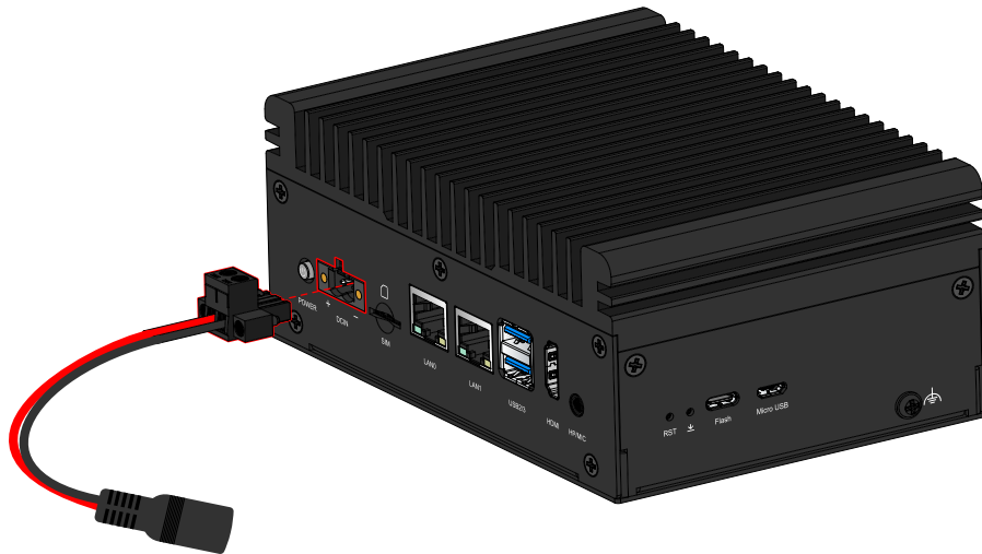
Figure 09: Connecting the power cable to the system
