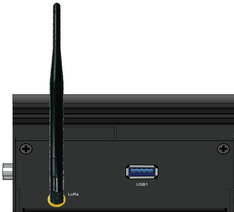
Figure 08: Installed LoRa antenna
