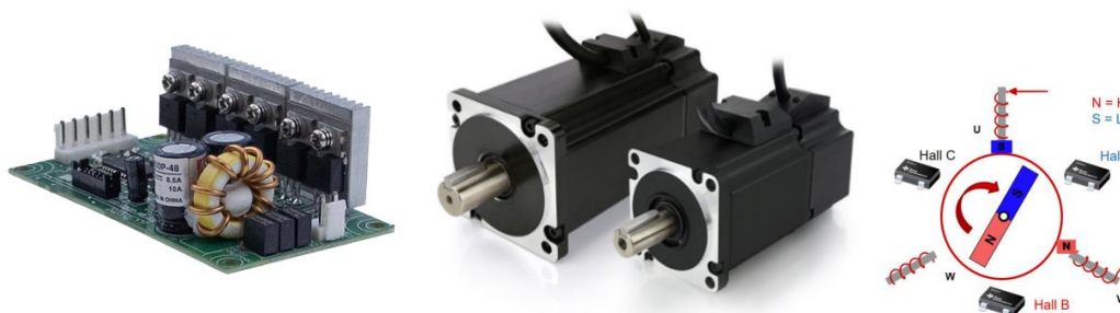
Figure 1. VFD module and Hall sensor BLDC motor
