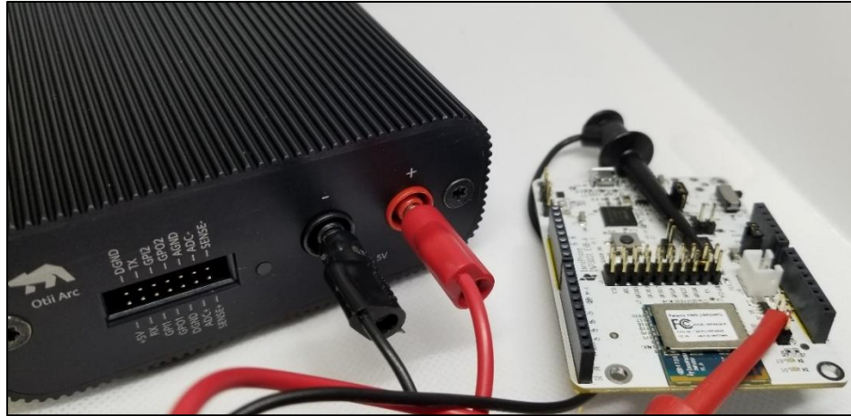
Figure 14: Current measurement setup using Otti Arc
