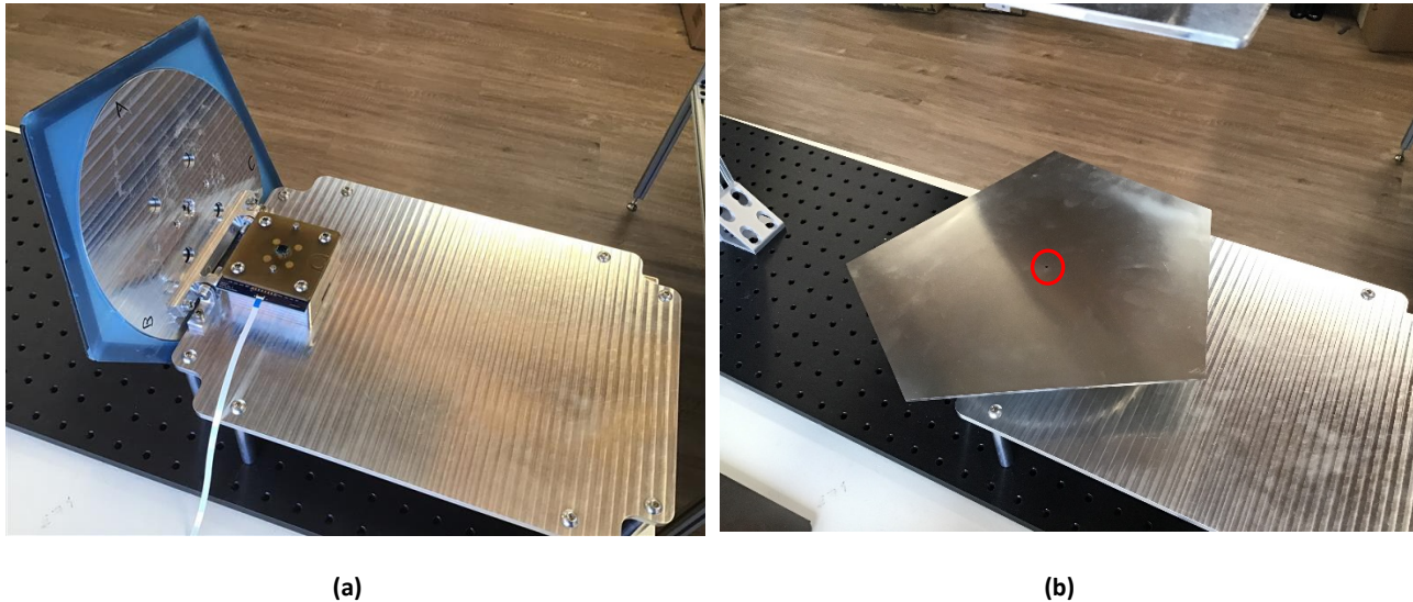
Figure 5 (a). Photograph showing the open baffle and test socket. A module has been placed in the test socket.
