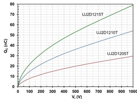
Fig. 2: Capacitive charges  $Q_c$  of USCi's 1200V SiC JBS diodes obtained by integrating the typical  $C_j$  vs.  $V_r$  curves.
