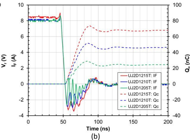
Fig. 6: Measured turn-off waveforms (a) and capacitive charge  $Q_c$  (b) of the 1200V SiC JBS diodes UJ2D1215T, UJ2D1210T, and UJ2D1205T at  $T_j = 25^\circ\text{C}$ . Switch: UJC1206K.
