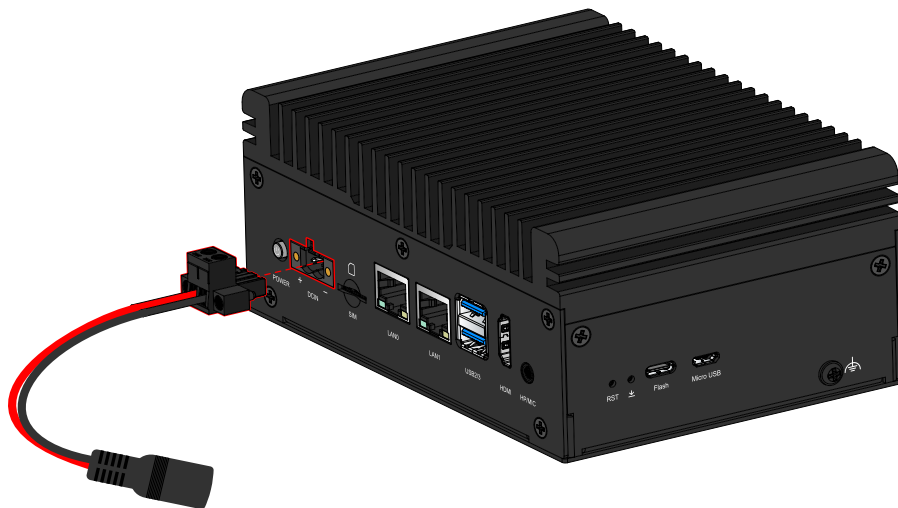
Figure 29: Connecting the power cable to the system
