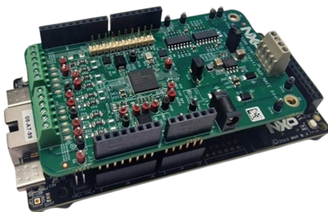
Figure 4. NAFE13388-UIM expansion board connected to the FRDM MCXN-947 evaluation board
