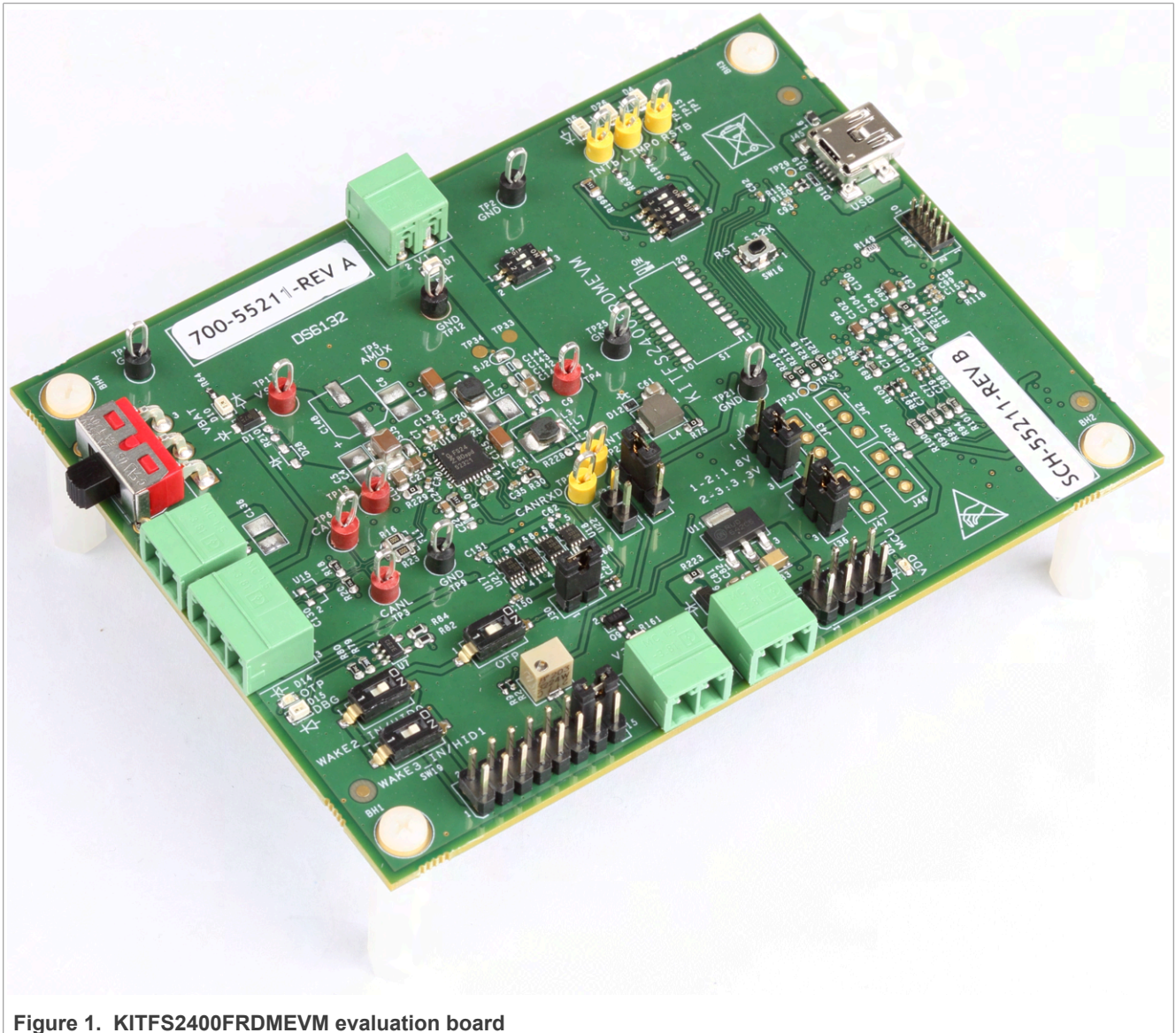
Figure 1. KITFS2400FRDMEVM evaluation board
