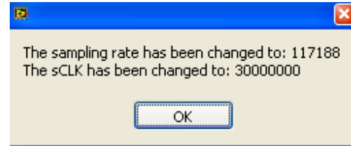
Figure 21. Software Overwritten User Settings to a Sample Rate/SCLK Rate Suitable for SDP Data Transfer
