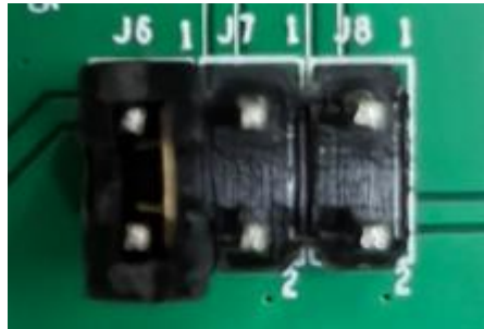
Figure 9: Switch used for power supply on JS-1125 EVB
