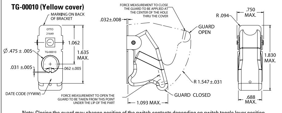
Note: Closing the guard may change position of the switch contacts depending on switch toggle lever position.
