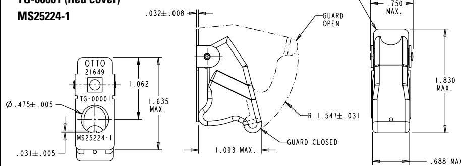
Note: Closing the guard may change position of the switch contacts depending on switch toggle lever position.
