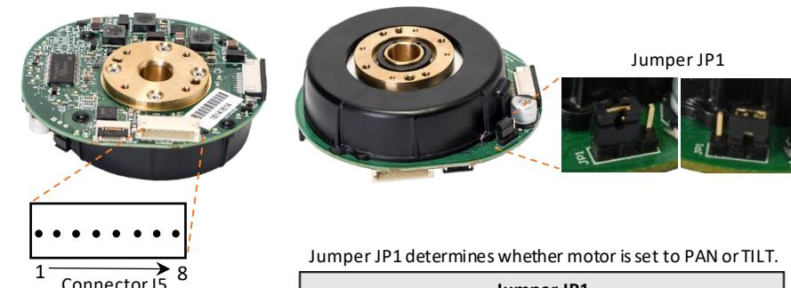
Jumper JP1 determines whether motor is set to PAN or TILT.
