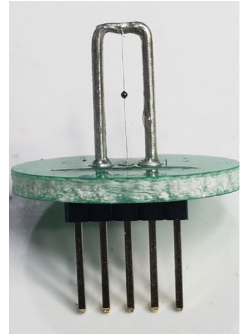
Sample of Blackbead welded to header
