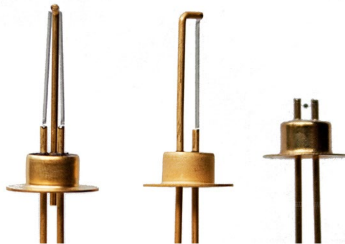
Sample of Blackbead welded to header
