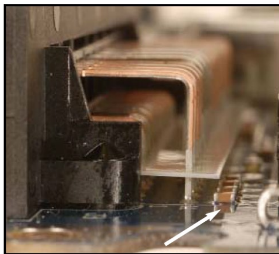
Figure 2 – Filter capacitor very near thru-hole connector.
