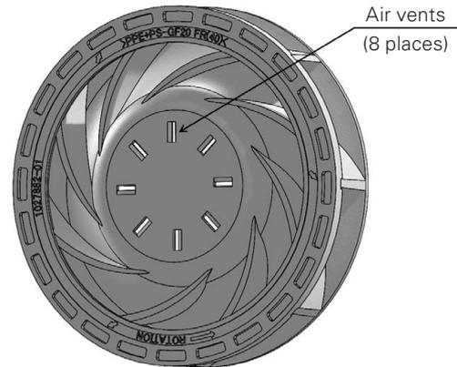
Fig. 6 Cooling structure of the new model
