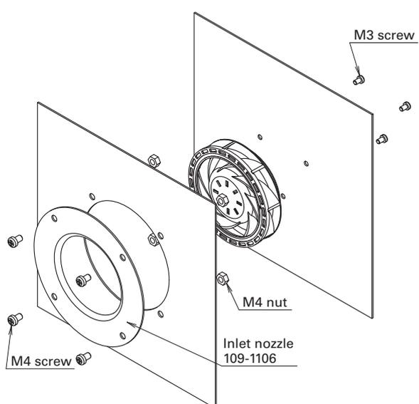
Fig. 3 Installation of inlet nozzle on new model
