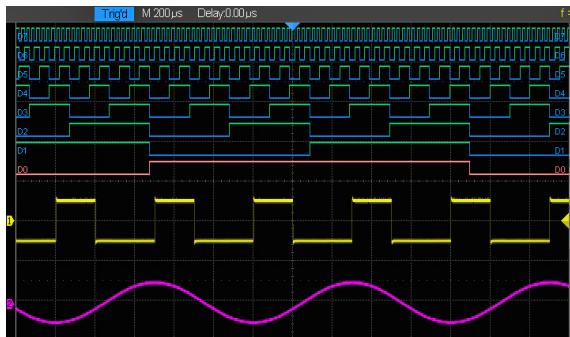
The MSO option adds 16 digital channels to the T3DSO3000 enabling users to trigger and acquire digital as well as analog waveforms in a mixed signal debug environment.
