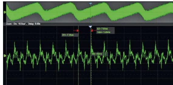
The record length of up to 250 Mpts (interleaved) or up to 125 Mpts (non-interleaved) allows use of a higher sampling rate to capture more signal detail. The hardware-based Zoom then allows quick zoom in to any area of interest.
