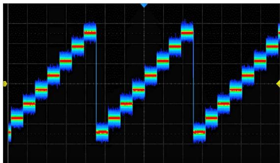
The Color temperature display clearly shows noise and jitter with infrequently occurring waveforms shown in blue through to the most frequently occurring waveforms shown in red.
