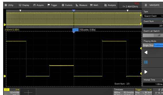
The T3DSO3000 can find events within an acquisition record or history acquisition based on user specified trigger conditions. Navigate browses through Events flagged by the Search, plays back history events or continuously moves the delay position on long records (very useful in zoom view).
