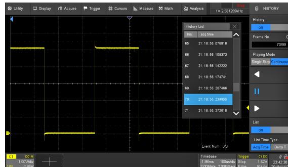
The always enabled History mode records up to 100,000 waveforms allowing users to scroll back through previous acquisitions to analyze past events and locate anomalies quickly. Serial decode, zoom and cursor measurements can be used.
