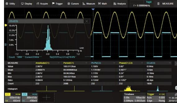
Parameter measurements include 4 categories: Vertical, Horizontal, Miscellaneous and Channel Delay providing over 50 different types of measurements.
