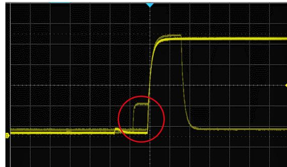
With a waveform capture rate of up to 500,000wfm/s (sequence mode) and 110,000 wfm/s (normal mode) the T3DSO3000 can easily capture glitches, infrequent anomalies and other low-probability events.
