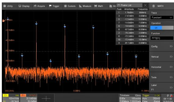
Two Math traces support Plus, Minus, Multiply, Divide, FFT, integration, differential, square root, and formula editor, providing a quick insight into the waveform characteristics.
