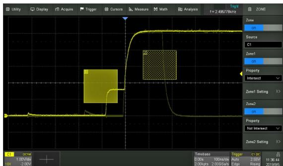
Set up to 2 zones defining each as either an Intersect or a Non Intersect. Trigger occurs when conditions are met. Zone Trigger helps to simplify advanced triggering.
