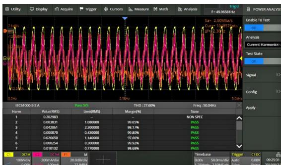
The T3DSO3000 Power Analysis application provides a full suite of power measurement and analysis tools. These tools enable an improvement in the efficiency of measurements made on switching power supplies and power devices. The Power Analysis application can measure Power Quality, Current Harmonics, Inrush Current, Switching Loss, Slew Rate, Modulation, Output Ripple, Turn On/Off, Transient Response, PSRR and Efficiency. Each measurement has a help screen showing a connection diagram with notes.
