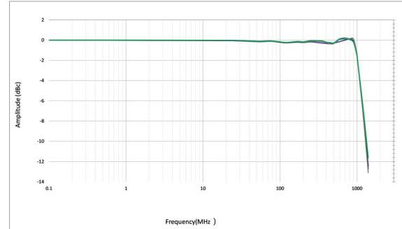
T3DSO31004 at 5 GSa/s shows exceptionally flat frequency response up to its maximum 1 GHz bandwidth.
