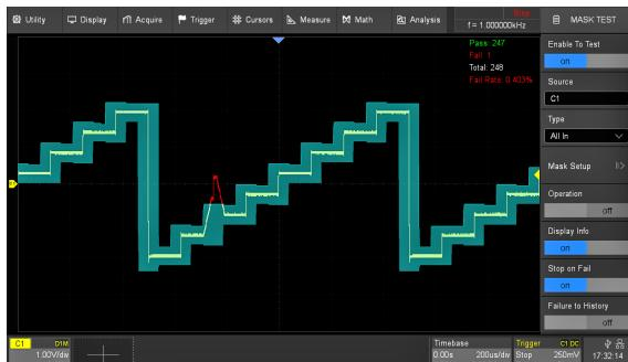
The T3DSO3000 utilizes a hardware based mask test function, that can perform 18,000 pass/fail tests per second. Users can define their own masks directly from a waveform or from the mask editor capability. The masks can then be used for Go/No Go testing with any failures stored as history waveforms or screen shots. The masks can also be stored on the T3DSO3000 for future use, making it suitable for long-term signal monitoring or automated production line testing.
