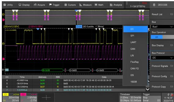
Simultaneously trigger and decode up to 2 common embedded and automotive serial buses, I<sup>2</sup>C, SPI, UART, LIN, CAN, CAN FD, FlexRay, I<sup>2</sup>S, MIL-STD-1553B, SENT and Manchester. Protocol information can be quickly and intuitively displayed, time aligned with the waveform and in table format.
