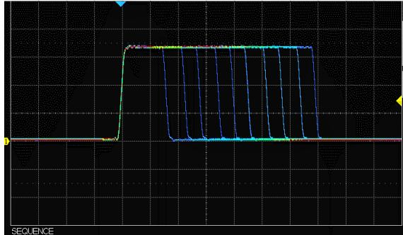
Segmented memory mode can store up to 100,000 waveforms into memory segments for capturing fast events in quick succession. Combine Sequence Mode with advanced triggers to isolate rare events. All the segments can be play back using the History function.
