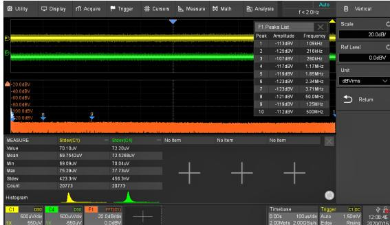
T3DSO31004: At 200 MHz bandwidth, the input noise floor is typically only 80  $\mu$ Vrms.
