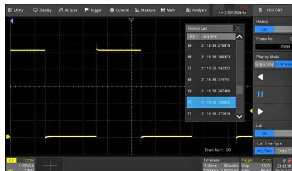
The always enabled History mode records up to 90,000 waveforms allowing users to scroll back through previous acquisitions to analyze past events and locate anomalies quickly. Serial decode, zoom and cursor measurements can be used.
