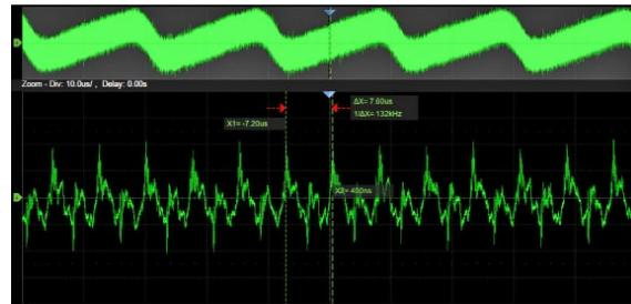
The record length of up to 200 Mpts (interleaved) or up to 100 Mpts (non-interleaved) allows use of a higher sampling rate to capture more signal detail. The hardware-based Zoom then allows quick zoom in to any area of interest.
