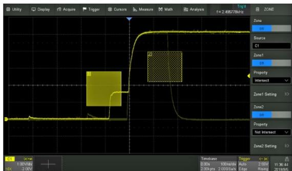
Set up to 2 zones defining each as Intersect or Not Intersect. Trigger occurs when conditions are met. Zone Trigger helps to simplify advanced triggering.
