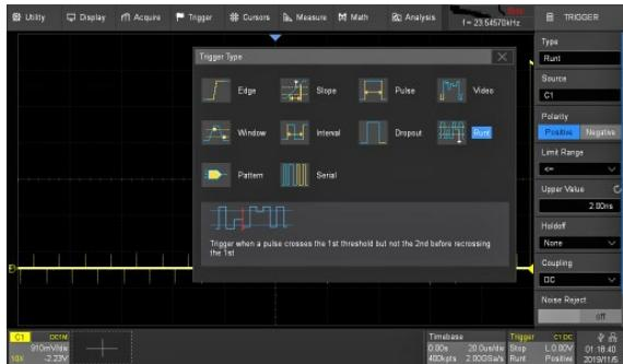
A wide range of powerful triggering functions including Edge, Slope, Pulse, Video, Window, Runt, Interval, Dropout, Pattern, Serial, etc, allows users to debug complex hardware issues with ease.
