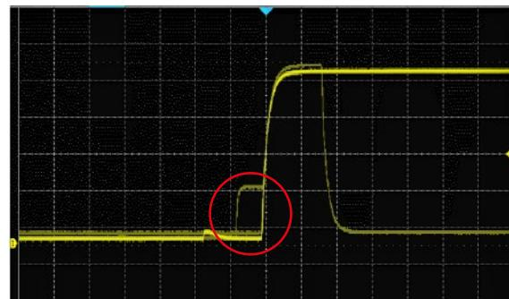
With a waveform capture rate of up to 500,000 wfm/s (sequence mode) and 120,000 wfm/s (standard mode) the T3DSO2000A can easily capture glitches, infrequent anomalies and other low-probability events.
