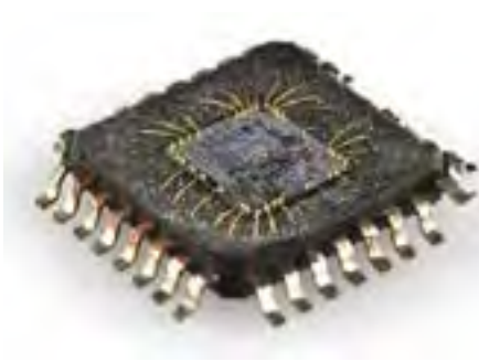
The guts of an integrated circuit, visible after removing the top.
