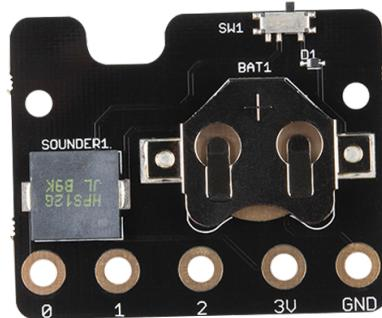
The Kitronik MI:power Board V2 has an easy-to-access on/off switch, which makes it easy to turn a project on and off, rather than have to disconnect the power supply from the BBC micro:bit. The kit contents include the MI:power board for the BBC micro:bit, three counter sunk M3 machine screws, three M3 Hex full-width nuts, three plastic spacers, and a CR2032 3V coin cell.
