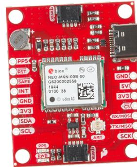
The NEO-M9N GPS Breakout is also equipped with an onboard rechargeable battery that provides power to the RTC on the NEO-M9N. The u-blox receiver supports I<sup>2</sup>C, making it ideal for Qwiic compatibility. The module detects jamming and spoofing events and can report them to the host, so the system can react to such events.
