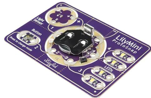
The LilyMini ProtoSnap comes with a pre-loaded code that uses all the LilyPad pieces connected to it. This sample code has three modes, which can be operated by selecting the LilyPad bottom on the bottom-left side of the ProtoSnap. The built-in RGB LED on the LilyMini will change color to indicate which mode has been selected. The white color indicates all LEDs are on, the cyan color signifies LEDs are switched off.
